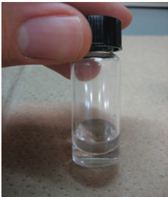
Figure 2 Photograph showing the immiscibility between PMMA solution and mineral oil. A distinct layer of mineral oil was found above the PMMA solution. [Color figure can be viewed in the online issue, which is available at www.interscience.wiley.com .]
